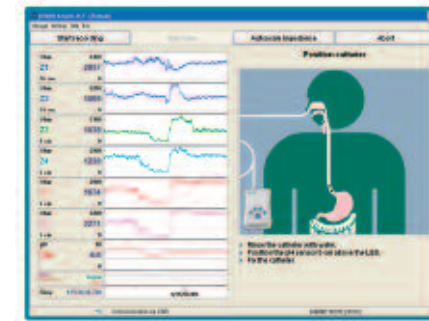
4. Position pH sensor (normally 5 cm above the LES). Instruct the patient on the use of recorder and send them away for the duration of the study.
